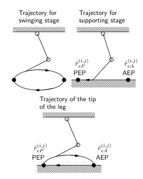
Fig. 3: Nominal trajectory of the tip of the leg
