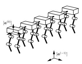
Fig. 1: Schematic model of a multipod robot The state variable is defined as follows;
